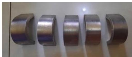
**Figure 7.** Raw Material Specimens After Being Given Bending Test
