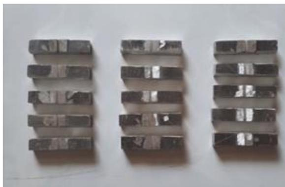
Figure. 1. Impact Test Specimens
