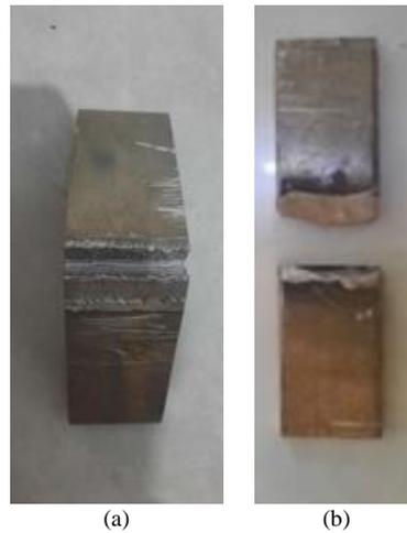
**Figure. 10.** (a) FSW Specimens After Being Given Bending Test. (b) TIG Specimens After Being Given Bending Test
