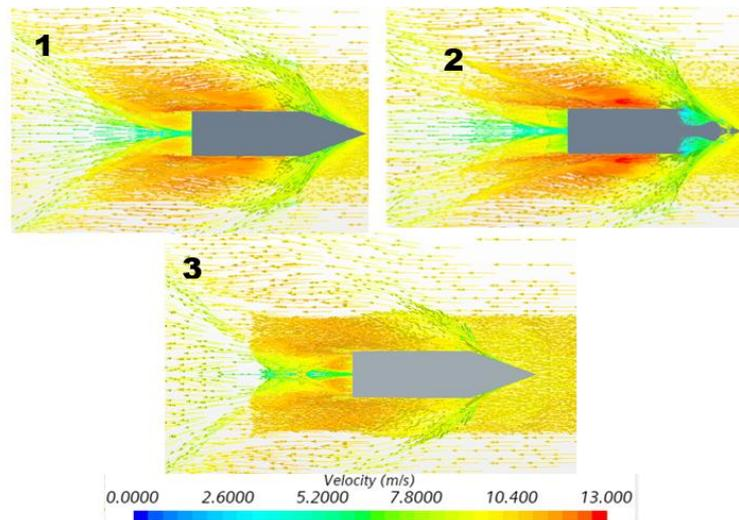
**Figure 7.** Velocity vector of the base model in three different Froude number model (1) base model, (2) hull vane model, (3) bow foil model on Froude number 0.59
