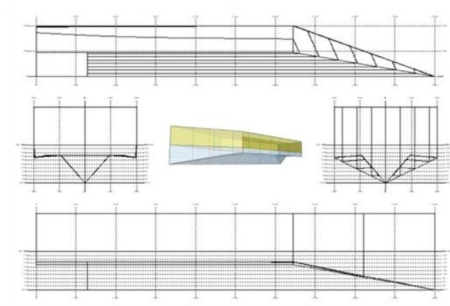
Figure 2. Ship geometry of flat-hull hull form ship
