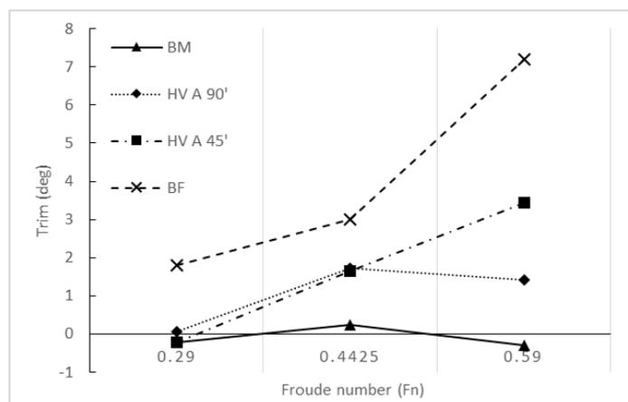
**Figure 8.** Trim value of 4 different conditions of flat-hull hull ship with a straight line (-) as the base model, dashed line (--) as bow foil model, dash-dot line (-.-) as hull vane model with 45° strut, and dot line (···) as hull vane model with 90° strut as a function of 3 different Froude number (0.29, 0.443, 0.59)
