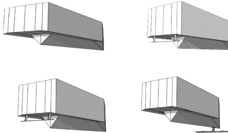
Figure 1. Ship geometry of flat-hull ship with different configuration foil
