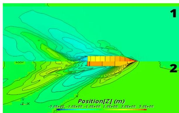
**Figure 5.** The wave pattern of the base model (1) and bow foil (2)
