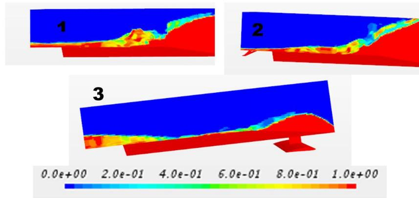
**Figure 6.** Trim visualization of the three variations of the ship model (1) base model, (2) hull vane model, (3) bow foil model on Froude number 0.59
