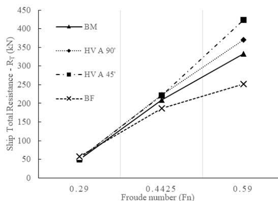
**Figure 4.** Total resistance ( $R_T$ ) of 4 different conditions of flat-hull hull ship with a straight line (-) as a base model, dashed line (--) as bow foil model, dash-dot line (-.-) as hull vane model with  $90^\circ$  strut and dot line (··) as hull vane model with  $45^\circ$  strut as a function of 3 different Froude number (0.29, 0.443, 0.59)
