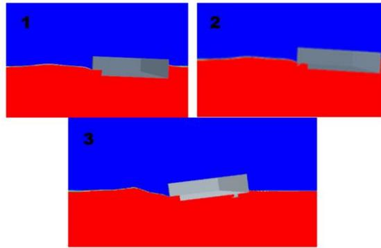
**Figure 9.** Trim visualization on the three variations of the ship model (1) base model, (2) hull vane model, (3) bow foil model on Froude number 0.59
