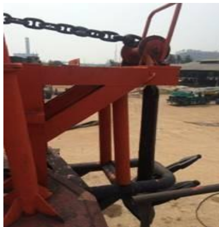
Figure 5. The position of the anchor stands upright
