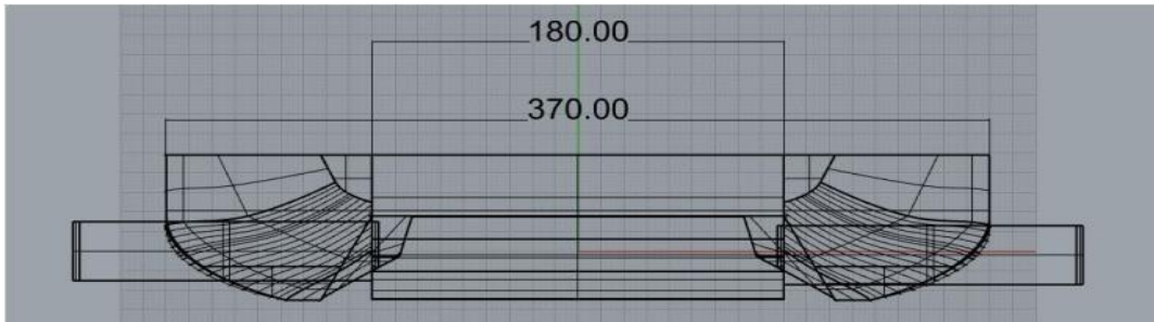
Figure 3. Winged conveyor with solid wings
