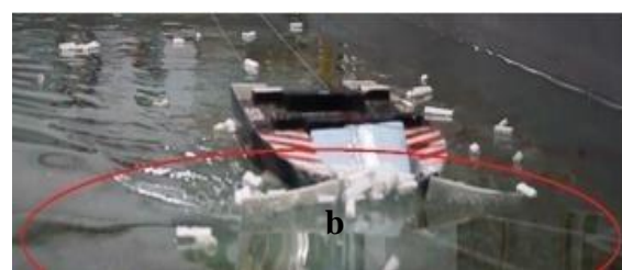
Figure 24: Water flow at 0.514 m/s (1 knot) (a) Ansys fluid fluent (b) experiment [14].
