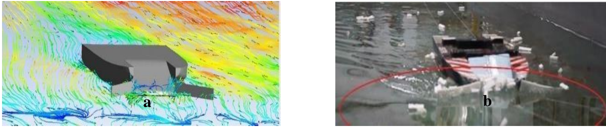
Figure 25: Water flow at 1.028 m/s (2 knots) (a) Ansys fluid fluent (b) experiment [14].
