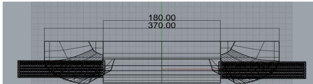
Figure 5. Winged conveyor with circle hole wing
