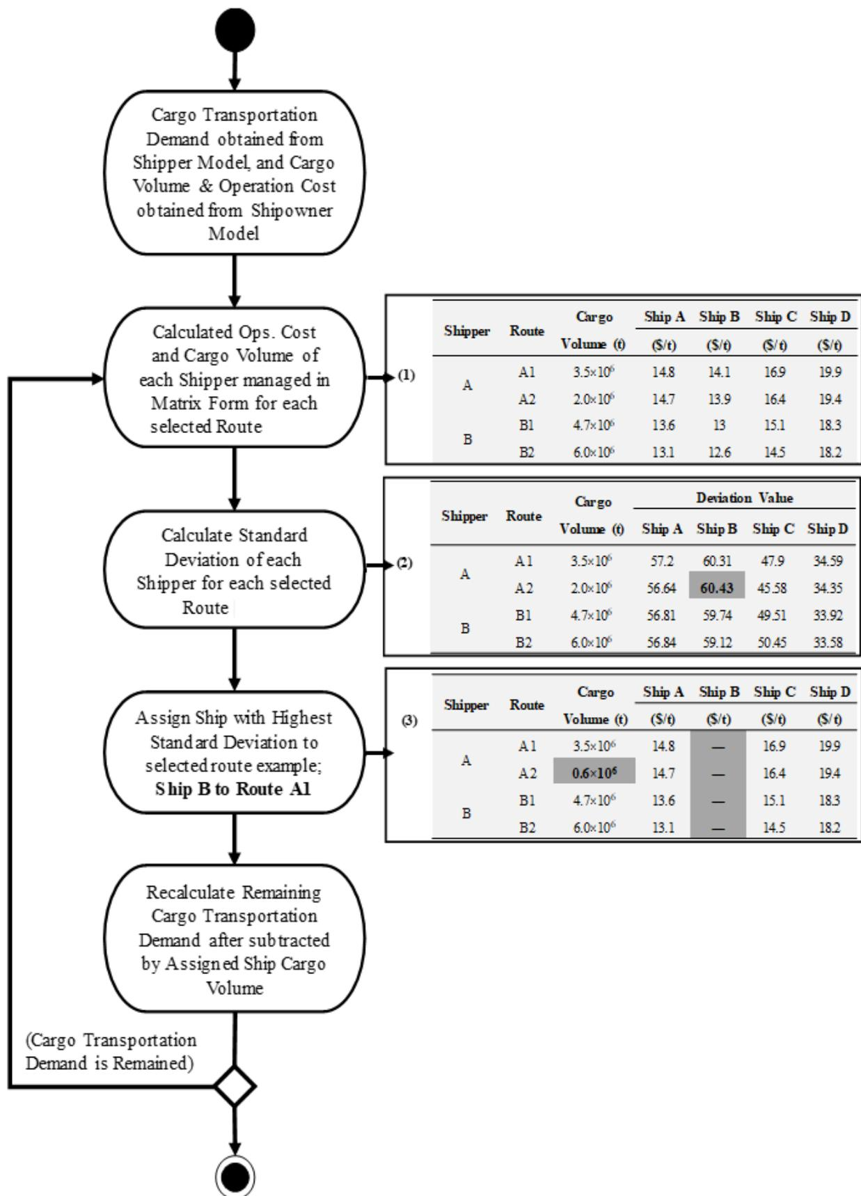
Figure 9. Operator Model
