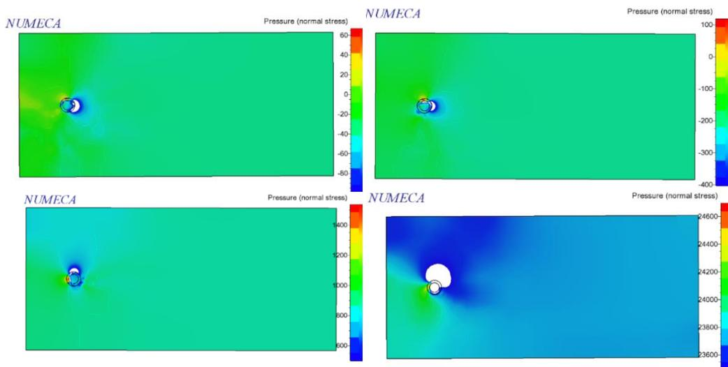
Figure 12 Pressure at Wind speed 10,20,30,35 [m/sec] with 150 RPM rotor speed for Model 2.
