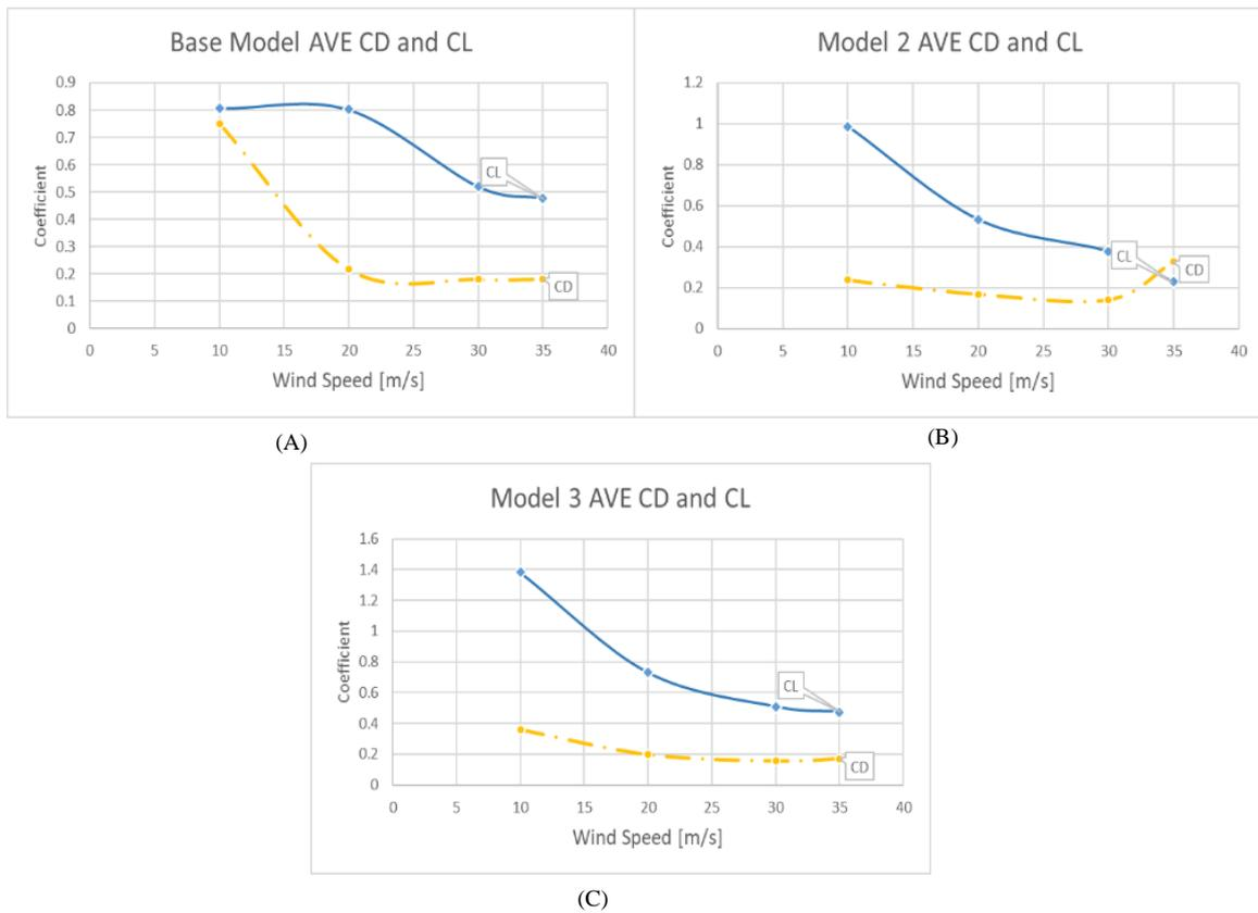
Figure 6 Average Lift and Drag Coefficients.
