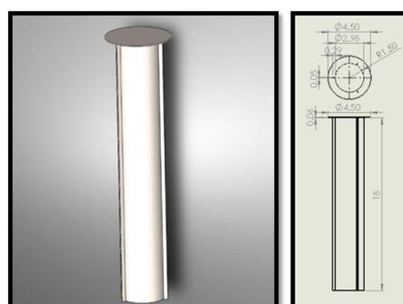
Figure 2 Flettner modified model1 and dimensions [m]
