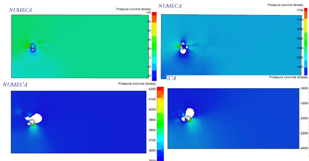
Figure 13 Pressure at Wind speed 10,20,30,35 [m/sec] with 50 RPM rotor speed for Model 3.
