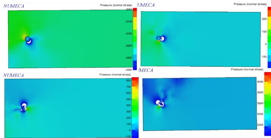
Figure 9 Pressure at Wind speed 10,20,30,35 [m/sec] with 150 RPM rotor speed for Base Mod
