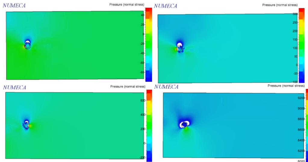
Figure 11 Pressure at Wind speed 10,20,30,35 [m/sec] with 100 RPM rotor speed for Model 2.
