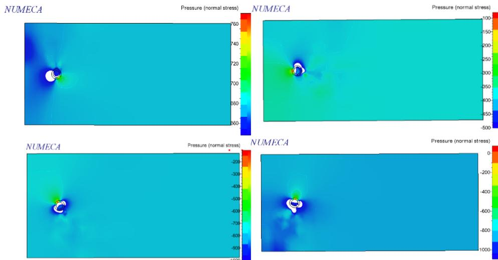
Figure 7 Pressure at Wind speed 10,20,30,35 [m/sec] with 50 RPM rotor speed for Base Model.
