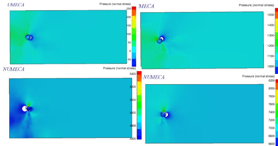
Figure 15 Pressure at Wind Speed 10,20,30,35 [m/sec] with 150 RPM rotor speed for Model 3.
