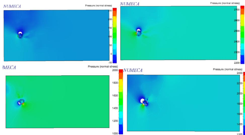
Figure 14 Pressure at Wind speed 10,20,30,35 [m/sec] with 100 RPM rotor speed for Model 3.
