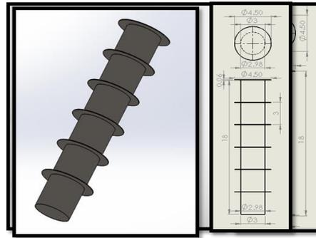
Figure 3 Flettner modified model 2 and dimensions [m].
