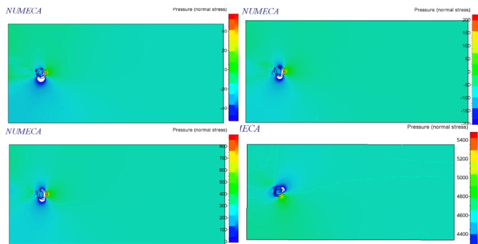
Figure 10 Pressure at Wind speed 10,20,30,35 [m/sec] with 50 RPM rotor speed for Model 2.
