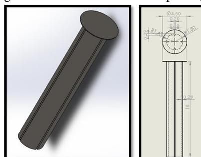
Figure 4 Flettner modified model 3 and dimensions [m].
