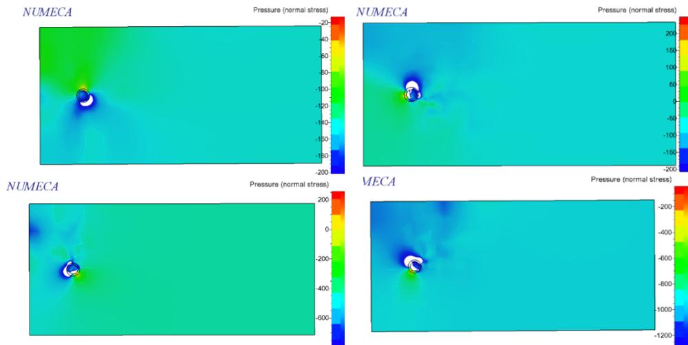
Figure 8 Pressure at Wind speed 10,20,30,35 [m/sec] with 100 RPM rotor speed for Base Model.
