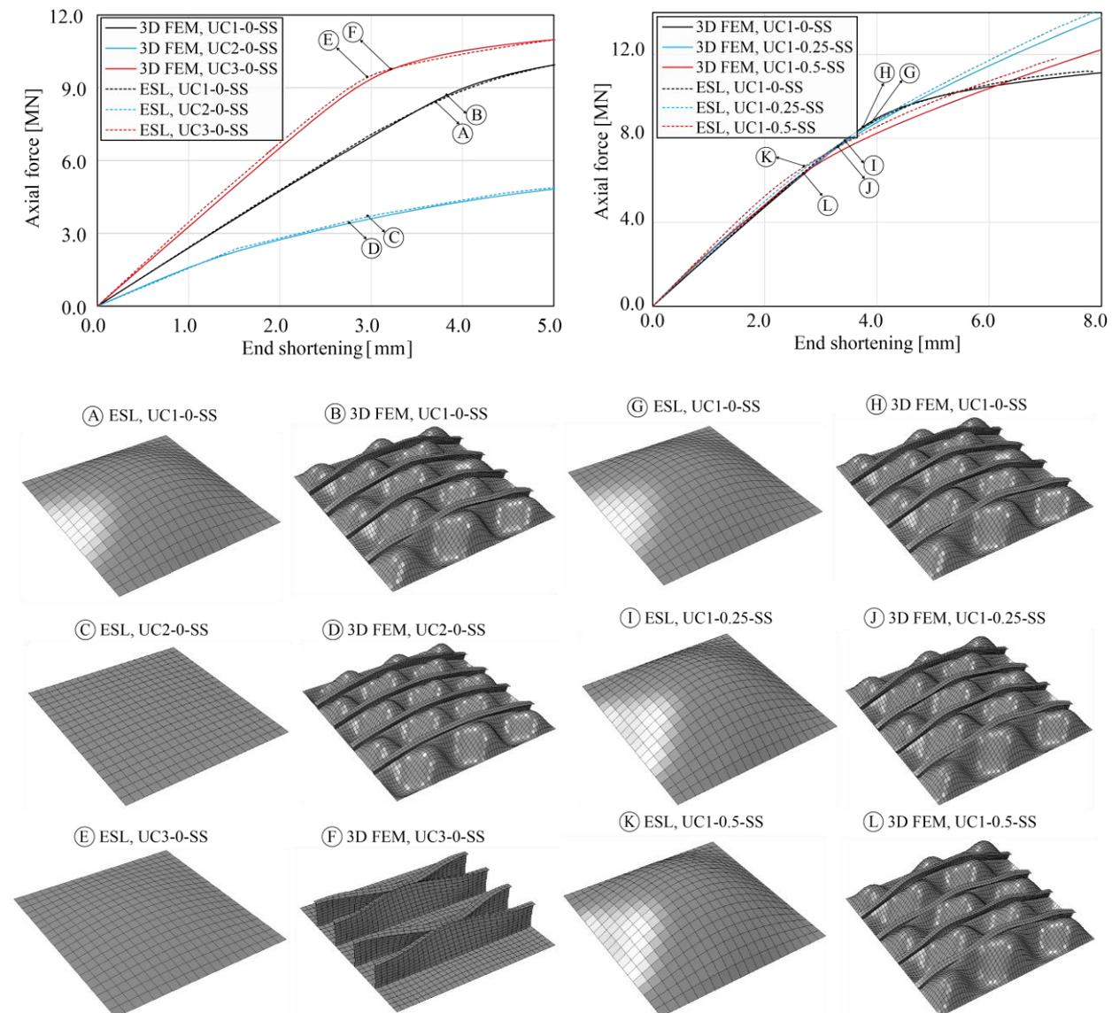
Figure 4. Load-end shortening curves and deformed shapes for UC1, UC2, and UC3 using simply supported boundary condition.
