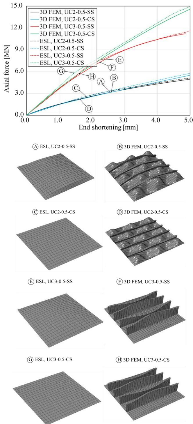
Figure 5. Load-end shortening curves and deformed shapes for biaxial compression using simply and clamped supports BCs.
