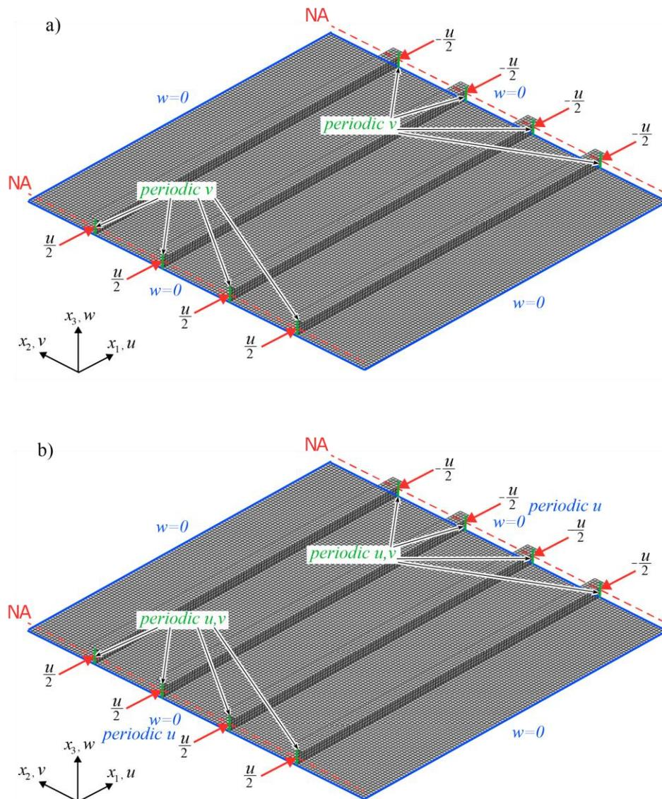
Figure 2. a) Simply supported and b) clamped boundary conditions applied in 3D stiffened panel for uniaxial compression. For biaxial compression, the displacement is added in the nodes of plate edges that perpendicular with the  $x_2$  direction.
