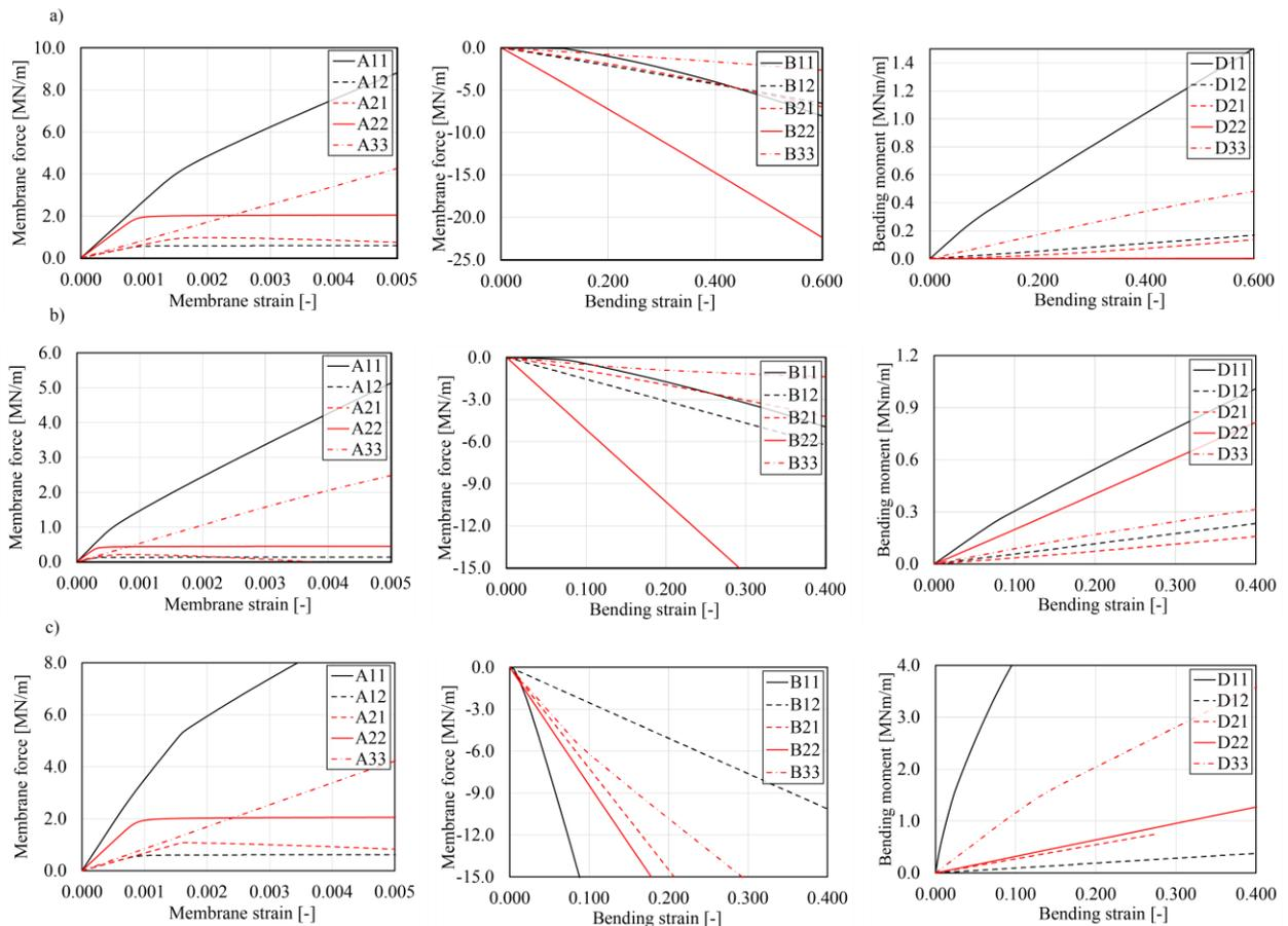
Figure 3. Non-linear stiffness of ESL for a) UC1, b) UC2, and c) UC3.
