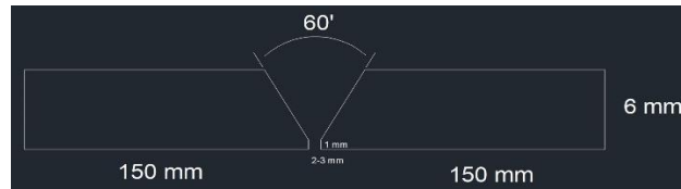
Figure 3. Welding joint design
