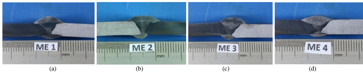
Figure 6. Macro metallographic test results (a) Specimen 1, (b) Specimen 2, (c) Specimen 3, (d) Specimen 4
