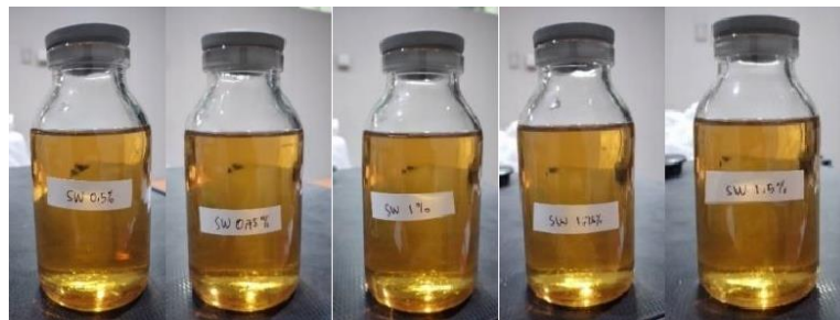
Figure 1. B30 after adding citronella oil at 0.5%, 0.75%, 1%, 1.25%, and 1.5% of the fuel volume.
