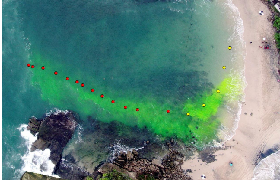
Figure 5. Measurements of rip current from uranine pigmented seawater on October 15 th 2022 at 10:50 am (local time); yellow and red dots represent feeder and neck, respectively, with interval time observation between adjacent dot is 15 second.
