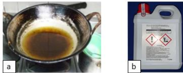
Figure 2. a) Raw Material: Used Cooking Oil. b) Cetane Number Improvement (2-Ethylhexyl Nitrate).
