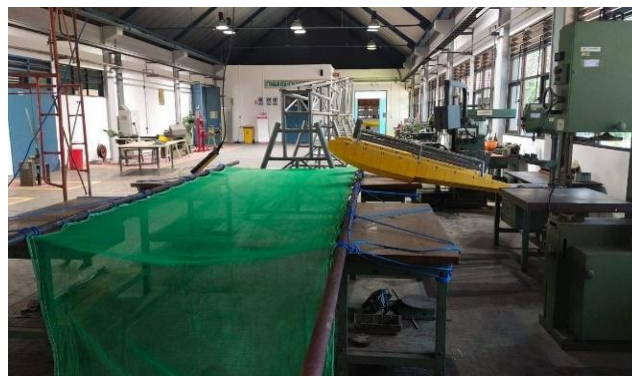
Figure 7. Placement of mesh nets in front of the launcher for securing the N219A floater model upon landing.
