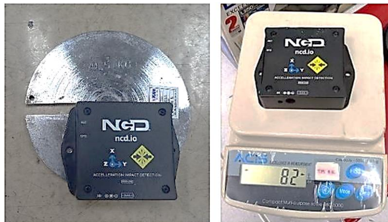
Figure 3. Weighting the sensor on scales
