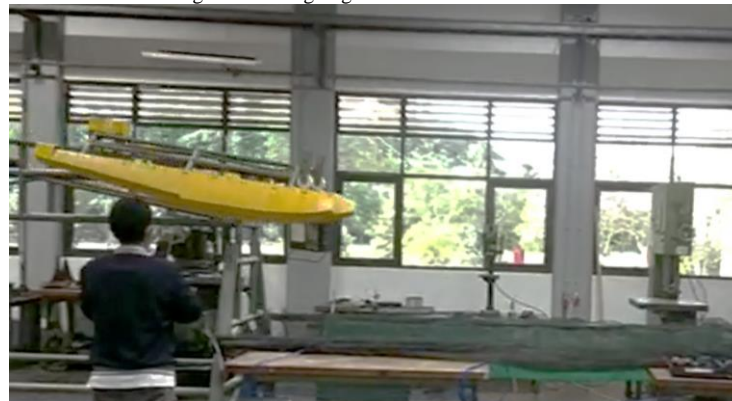
Figure 11. Time measurement of N219A floater model launching on the launcher until landing
