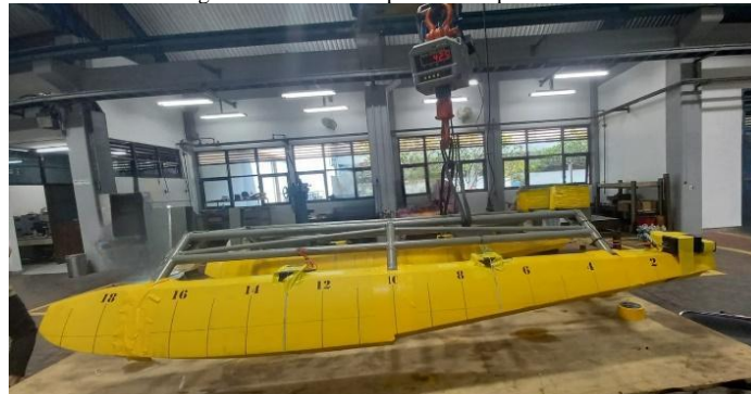
Figure 10. Weighing the N219A floater model.
