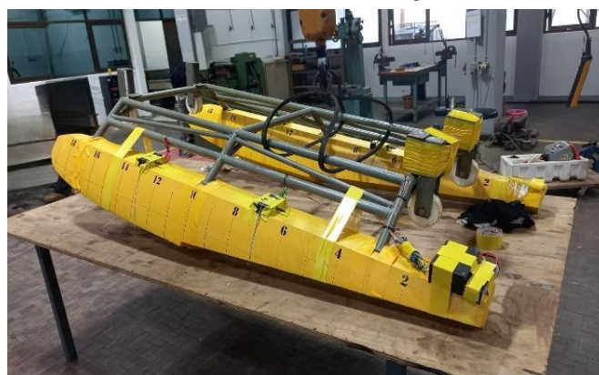
Figure 8. Placement of impact sensors and placement of ballast weights.
