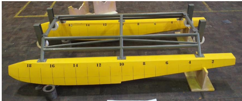
Figure 2. Model of the amphibious aircraft float
