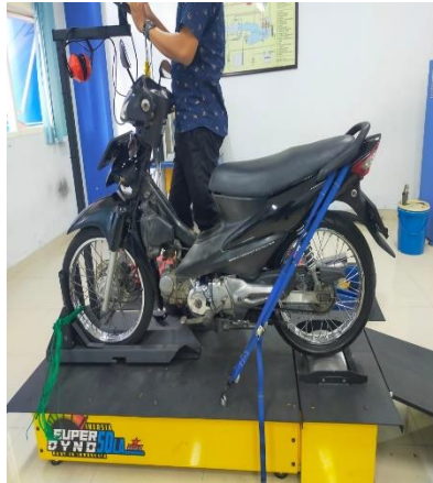
Figure 1. Testing scheme power and torque
