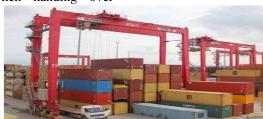
Figure 7 Rubber Tired Gantry (RTG)
