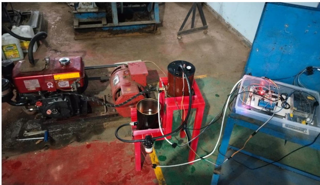
Figure. 2. B30 Bio Solar Fuel Heater Prototype Using Arduino
