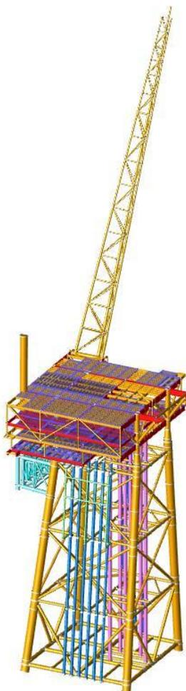
Figure 1. Jacket Structure Geometry Modeling Results.
