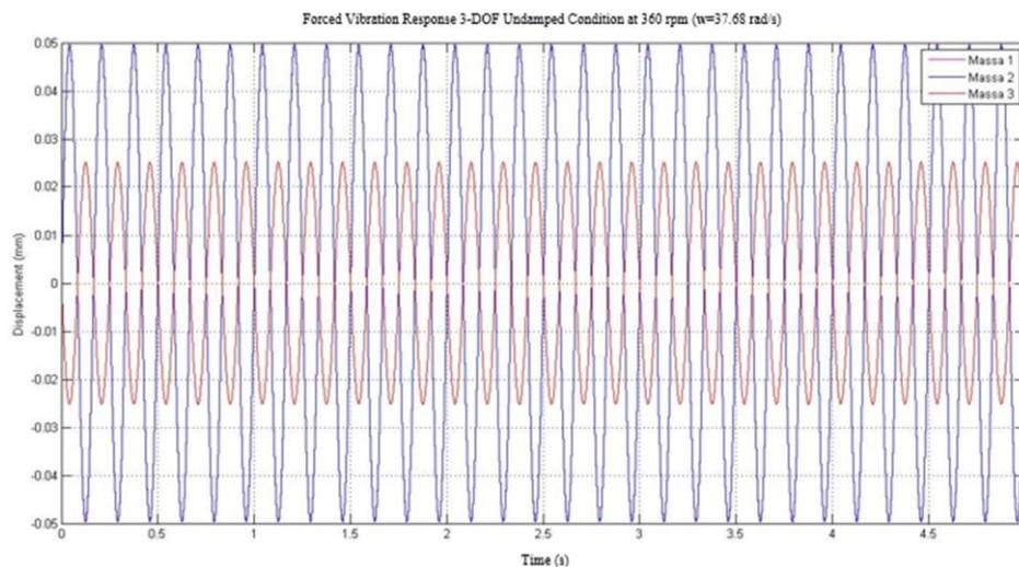
Figure. 7 . Graph of displacement response at 360 RPM.
