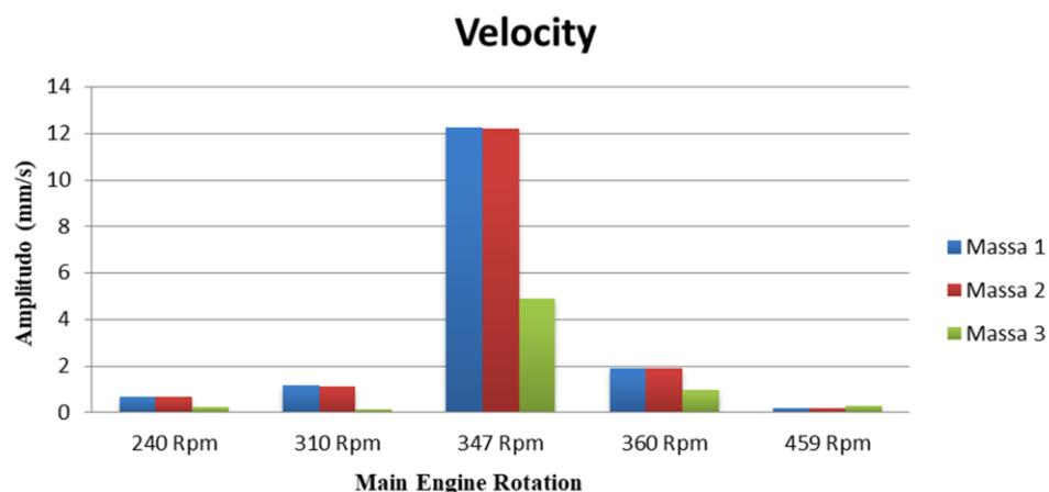
Figure. 15. Graph of velocity amplitude at variation of engine speed.
