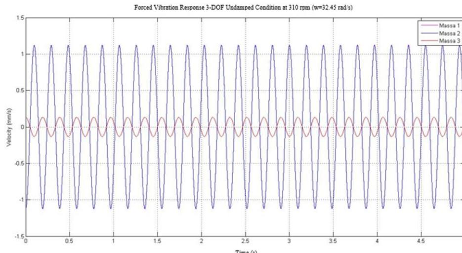
Figure. 10. Graph of velocity response at 310 RPM..
