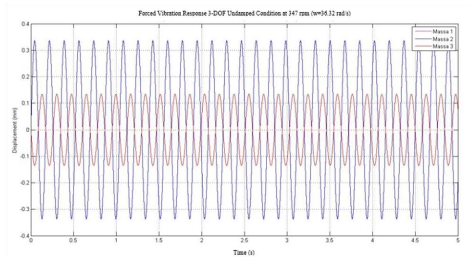
Figure. 6. Graph of displacement response at 347 RPM.
