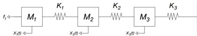
Figure. 1. Three-degree-of-freedom model of ship propulsion system.
