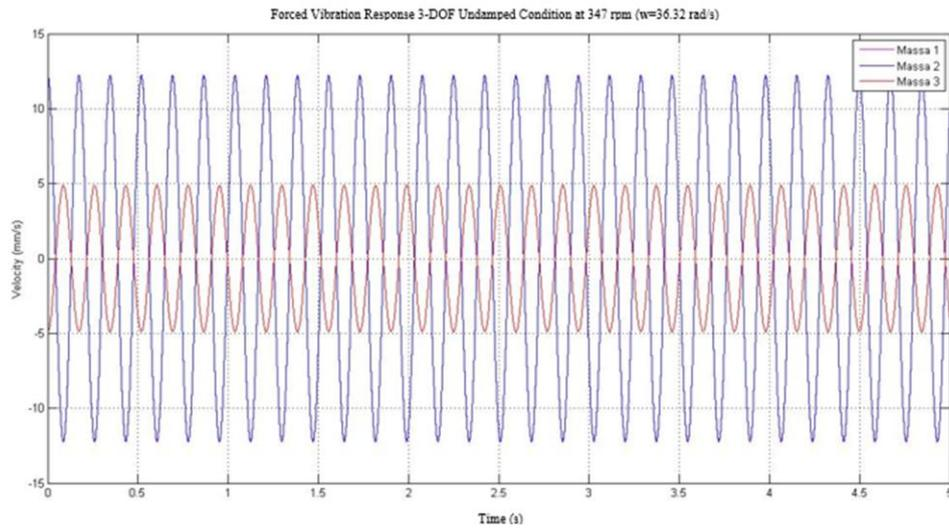
Figure 11. Graph of velocity response at 347 RPM..
