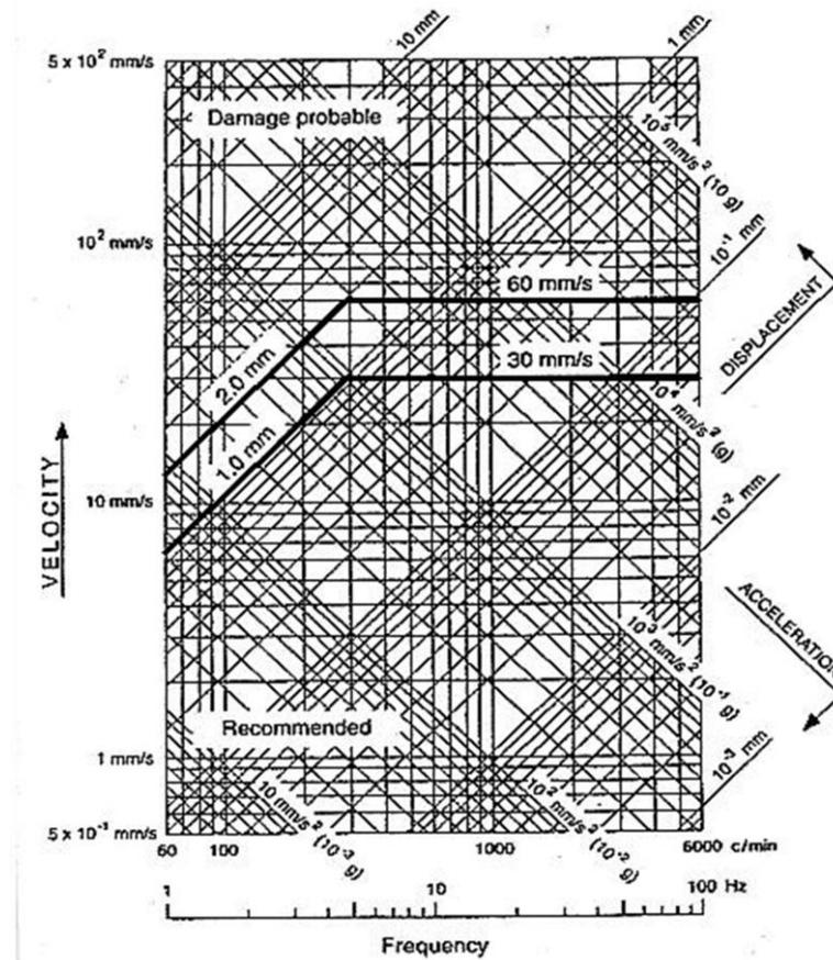
Figure 3. Vibration limitation by ABS.
