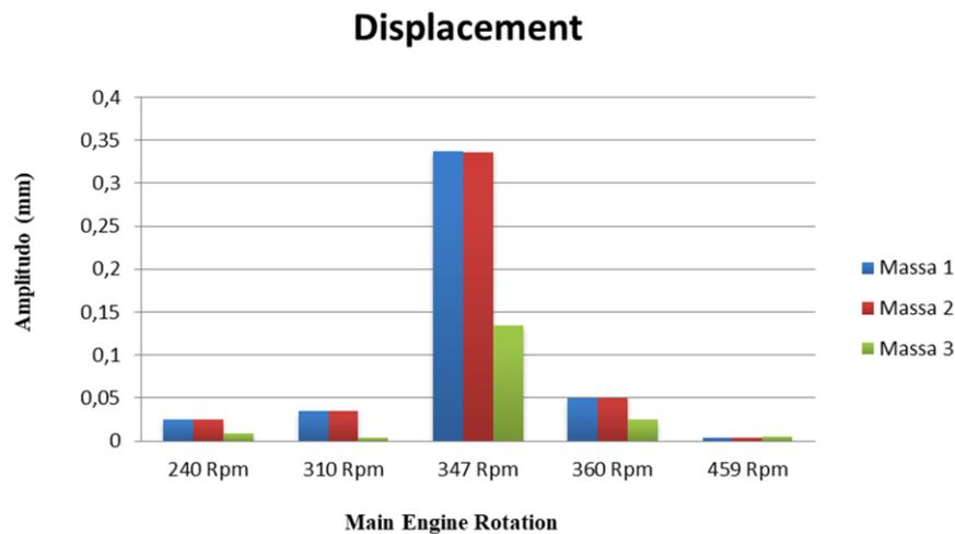
Figure. 14. Graph of displacement amplitude at variation of engine speed.
