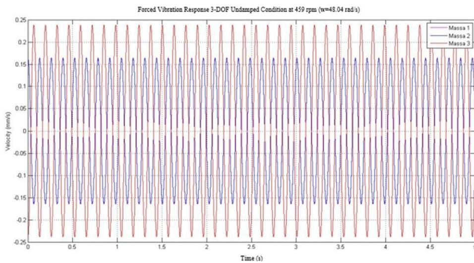
Figure 13. Graph of velocity response at 459 Rpm.
