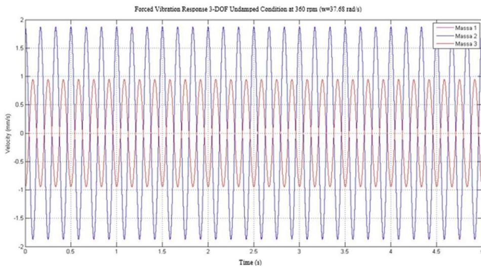
Figure 12. Graph of velocity response at 360 RPM..
