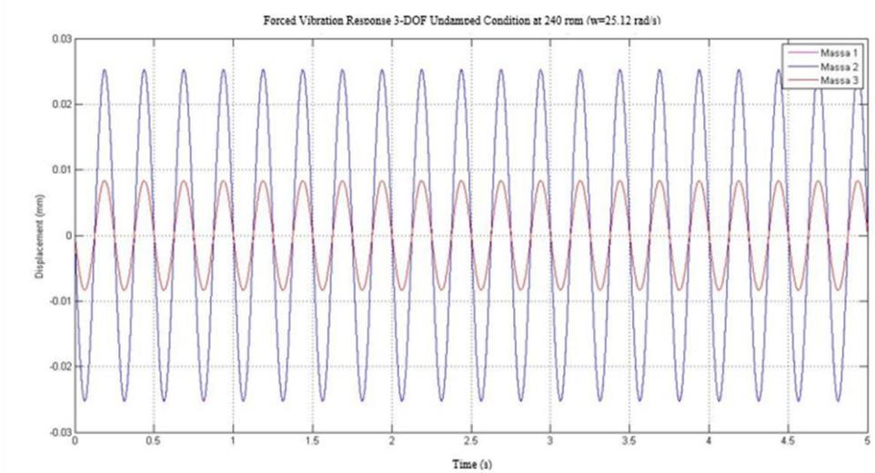
Figure. 4. Graph of displacement response at 240 RPM.
