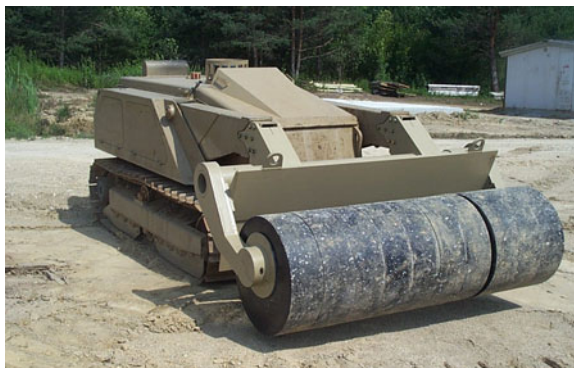
Fig. 2.30 Light demining machine with roller, 2t, 10 segments. (Reproduced with permission from Ref. [8])
