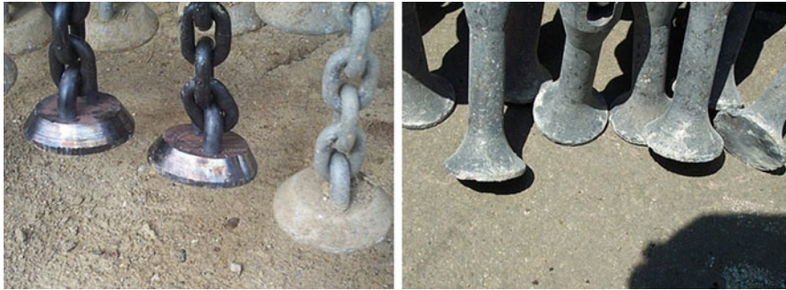
Fig. 2.16 Working shapes of striking hammers ( Source CROMAC-CTDT)
