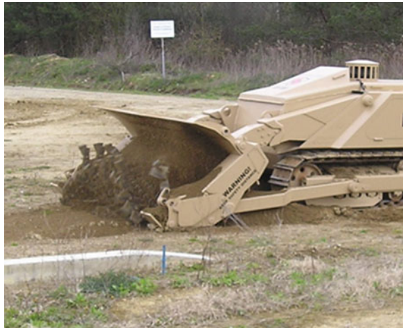
Fig. 2.25 Verification of a demining machine with tiller (Reproduced with permission from CROMAC-CTDT)
