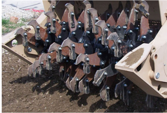
Fig. 2.24 Tiller working tool shape, wedge blade with “ears” (MV-4)
