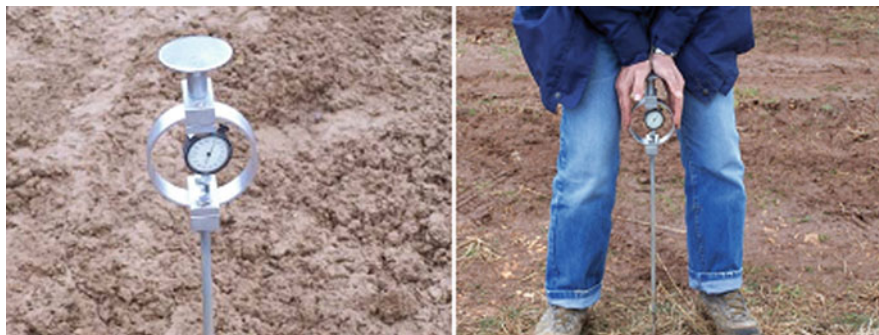
Fig. 2.1 Penetrometer for measuring the soil cone index
