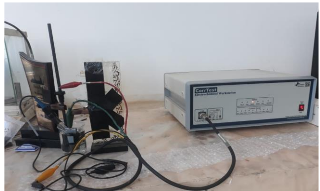
Figure 3. The Corrosion Rate Testing Process using 3 Electrode Cell Method
