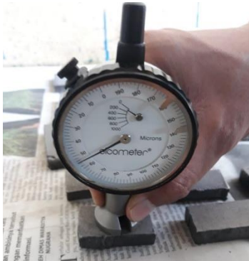
Figure 2. Surface Roughness Testing Process Specimens
