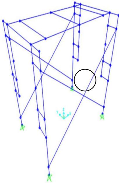
**Gambar 2.** *Scaffolding* 1 lantai tanpa *outrigger*
