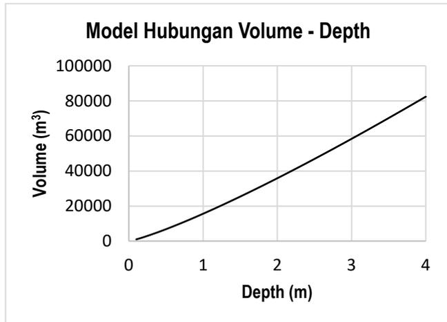
**Gambar 5.** Model Hubungan Volume-Depth
