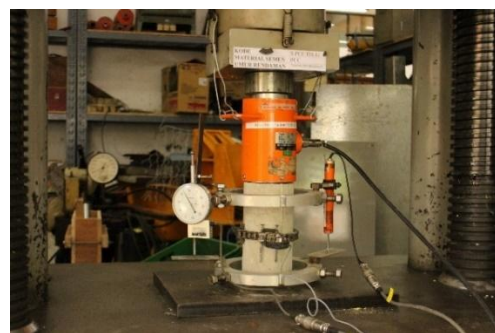
Figure 1 Testing setup of compressive strength, elastic modulus, and poisson's ratio
