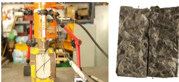
Figure 11 Damage visualization on splitting tensile strength test
