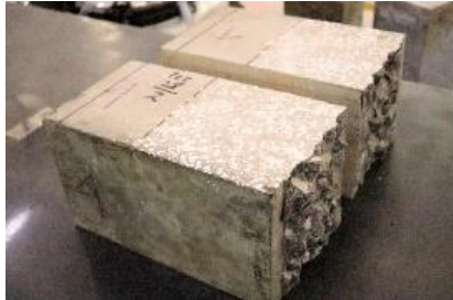
Figure 20 Damage visualization on fracture energy test
