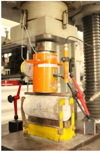
Figure 2 Testing setup of split tensile strength
