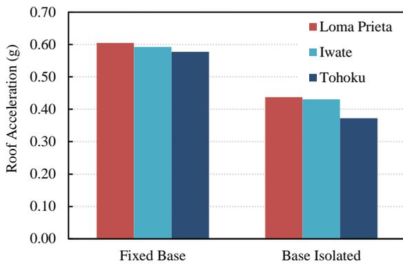
Figure 7 Comparison of roof acceleration in BSE-2E level
