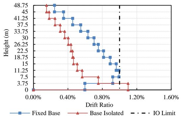
Figure 10 Comparison of interstory drift in BSE-1E level
