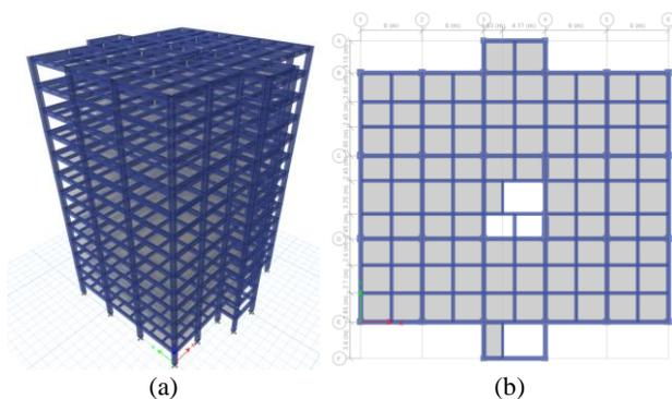
Figure 1 Numerical modelling of existing buildings: (a) 3D view, (b) Plan view
