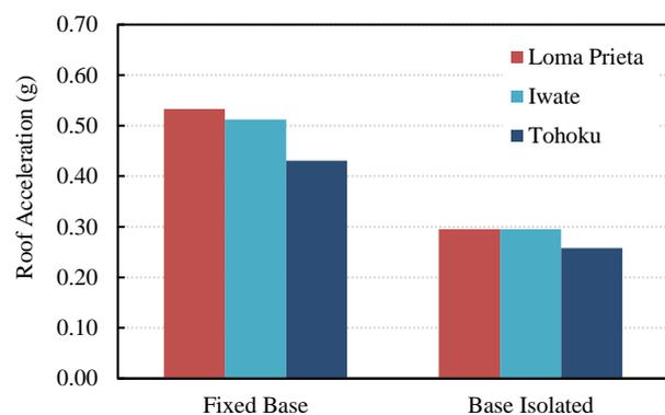
Figure 6 Comparison of roof acceleration in BSE-1E level
