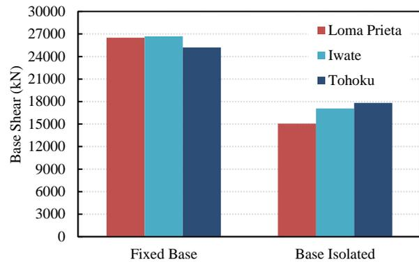
Figure 5 Comparison of base shear in BSE-2E level
