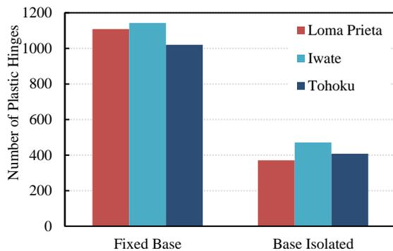
Figure 13 Comparison of number of plastic hinges formed in BSE-2E level
