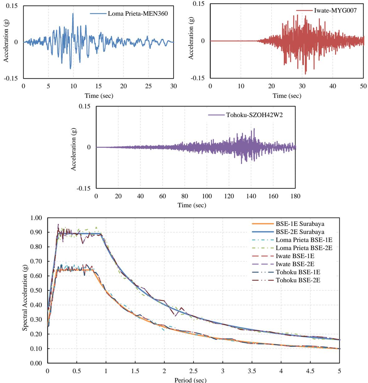
Figure 3 Spectrally matched ground motion records used for nonlinear time-history analysis: (a) Original accelerogram of three historical ground motion (b) Acceleration response spectra of the three ground motions matched to BSE-1E and BSE-2E level
