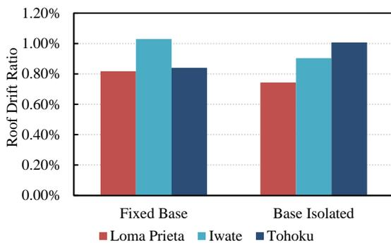
Figure 9 Comparison of roof drift ratio in BSE-2E level
