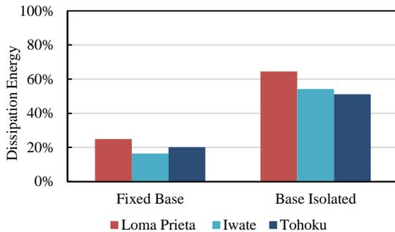
Figure 15 Comparison of dissipation energy in BSE-2E level
