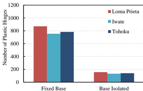
Figure 12 Comparison of number of plastic hinges formed in BSE-1E level
