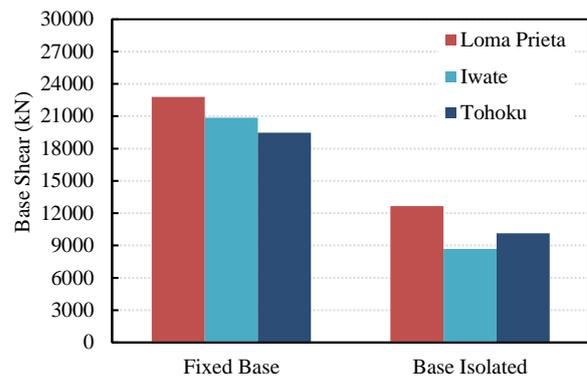
Figure 4 Comparison of base shear in BSE-1E level
