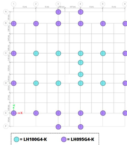
Figure 2 Isolator plan
