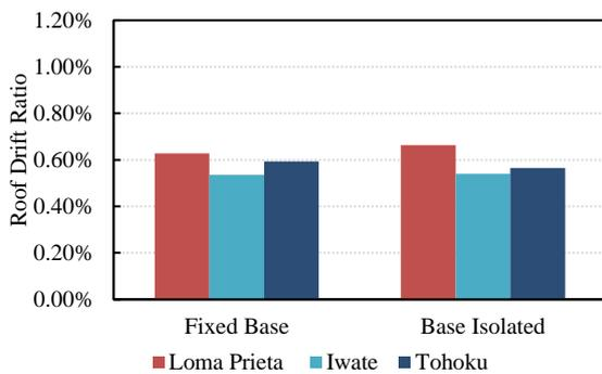
Figure 8 Comparison of roof drift ratio in BSE-1E level
