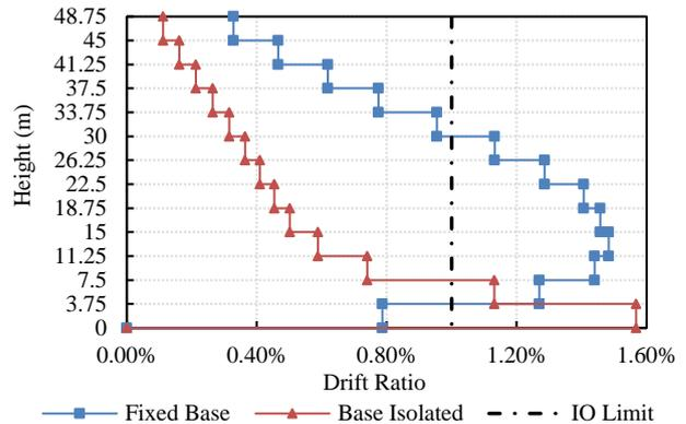
Figure 11 Comparison of interstory drift in BSE-2E level
