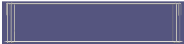
Figure 5 Rebar elements model UH5F1 specimen
