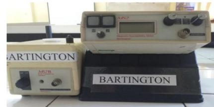
FIG. 3: Bartington Magnetic Susceptibility Meter MS2B sensor type at Geophysics Laboratory, Universitas Negeri Padang.
