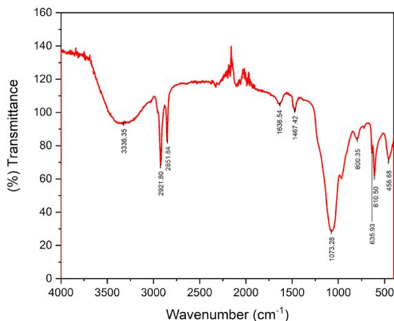
FIG. 1: FTIR spectrum of SiO<sub>2</sub> power from rice husk ash.
