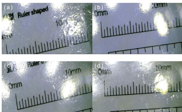
FIG. 3: Glass sample coated by modified SiO<sub>2</sub>/PDMS with various SiO<sub>2</sub> (a) 0.5 g, (b) 1 g, (c) 1.5 g, (d) 2 g.
