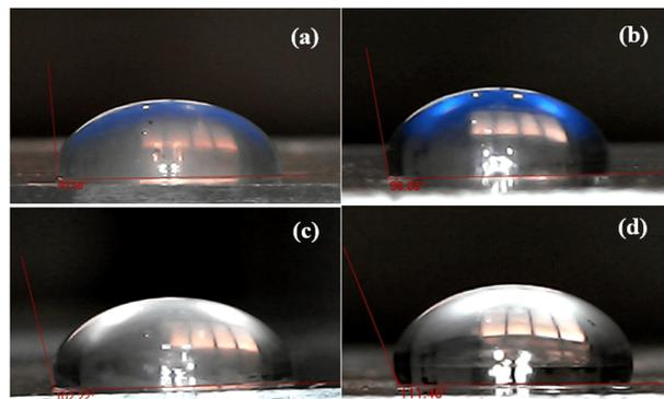
FIG. 4: Water contact angle of glass sample with coating PDMS/SiO<sub>2</sub> (a) 0.5 g (b) 1 g (c) 1.5 g (d) 2 g.
