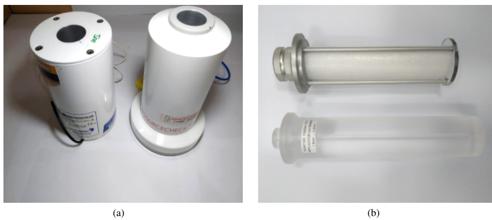
FIG. 2: (a) (left-side) Well-type chamber PTW SourceCheck 4, (right-side) Well-Type chamber HDR1000Plus (b) Adapter for transport tube.
