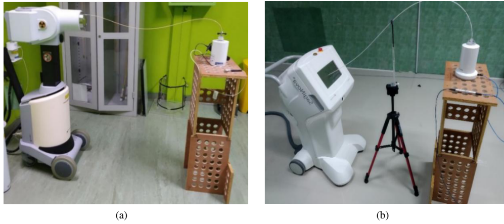
FIG. 1: Calibration setting on the custom wooden table and (a) Nucletron microSelectron afterloading machine (b) Gamma Med Plus IX afterloading machine.
