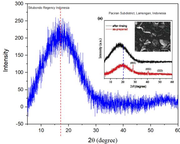
FIG. 1: XRD pattern of *a*-C powder derived from palmyra sugar obtained in Situbondo, inset showed the XRD pattern of palmyra sugar obtained from Paciran.
