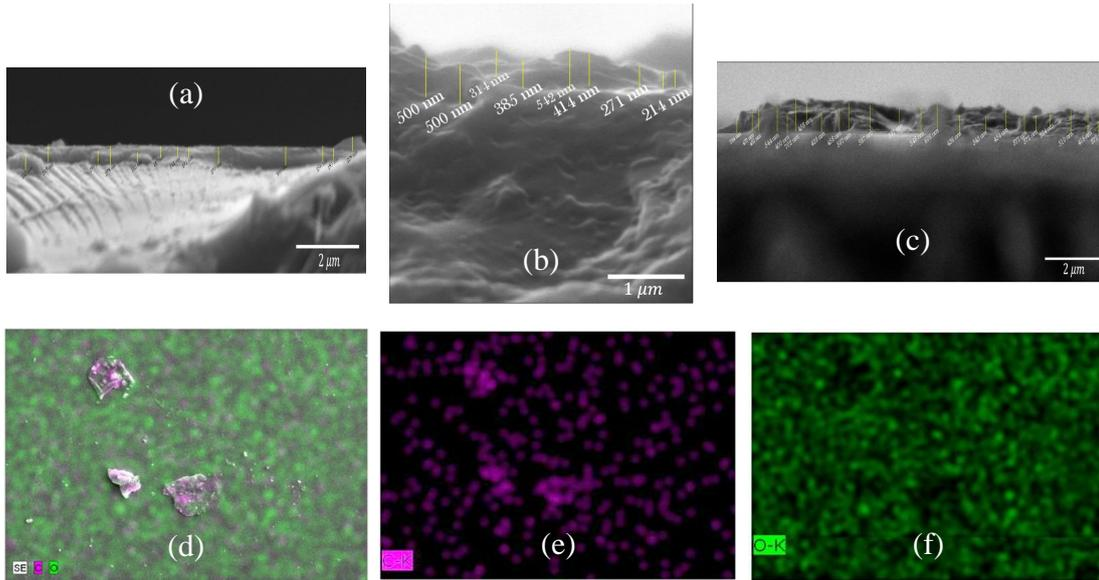
FIG. 2: SEM cross-section image of the *a*-C films prepared at the deposition time of (a)5 s, (b)20 s, (c) 25 s, (d) Elemental mapping of *a*-C films, showing the present of (e) carbon (C), (f) oxygen (O).
