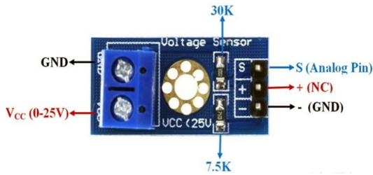
FIG. 2: Splitter sensor module pinout voltage [6]
