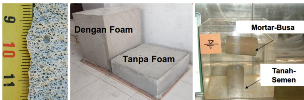
Figure 2. Foamed mortar lightweight mortar.
