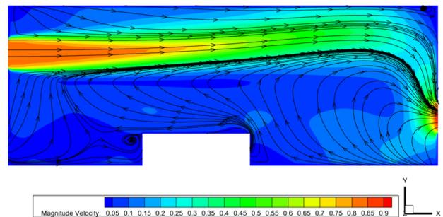
**Figure 5.** The contour of air velocity and streamline in a single bed isolation room in the x-y plane ( $z=3$ )
