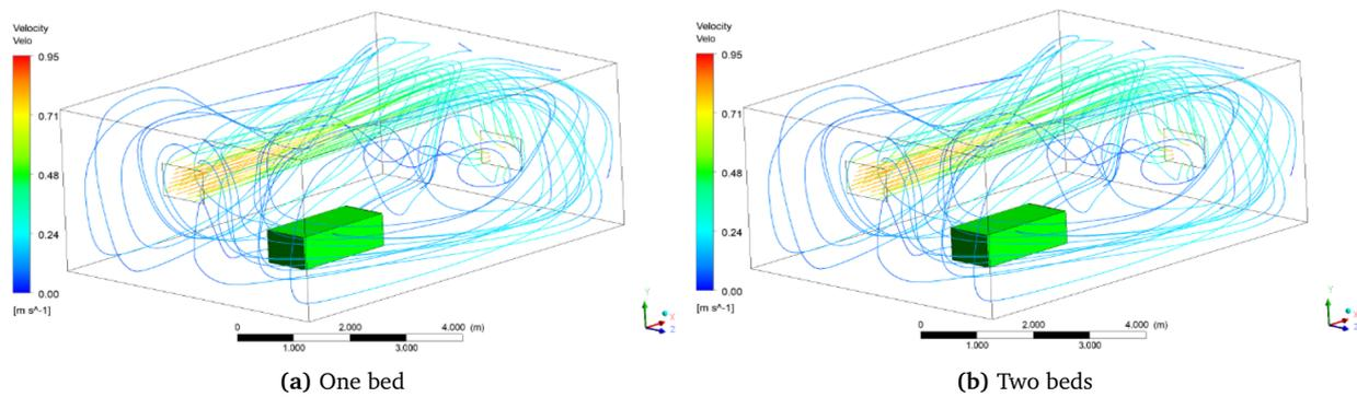
**Figure 4.** Velocity pathline in an isolation room with (a) one bed and (b) two beds
