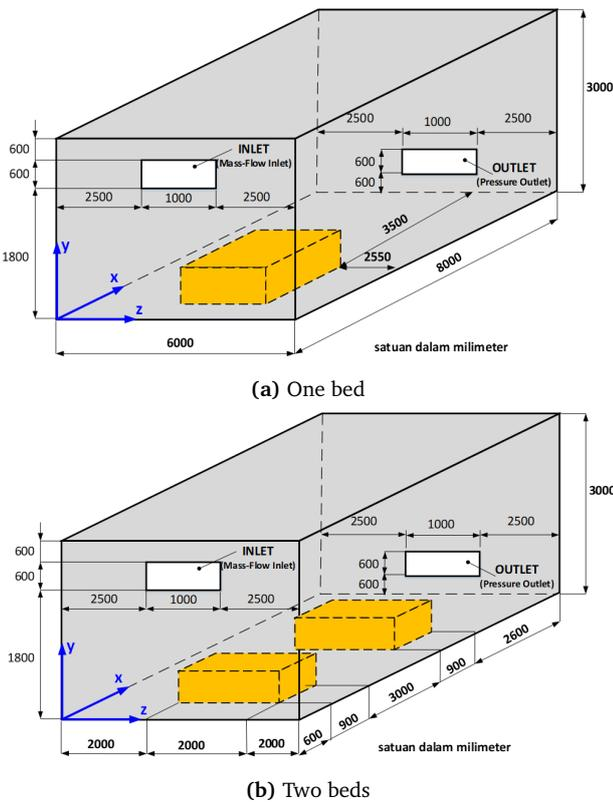
Figure 1. Schematic diagram of the isolation room with (a) one bed and (b) two beds
