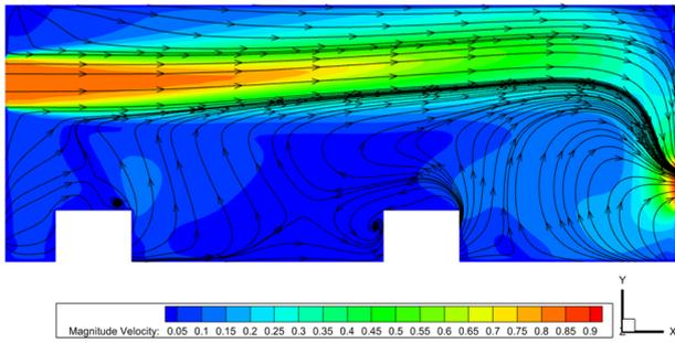
**Figure 7.** The contour of air velocity and streamline in a two-bed isolation room in the x-y plane ( $z=3$ )
