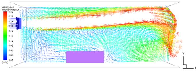
Figure 12. The flow vector in the one bed isolation room in the x-y plane ( $z=3$ )
