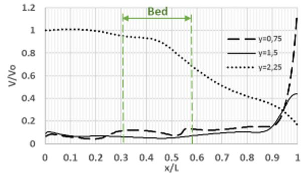
**Figure 10.** Graph of flow velocity distribution in a single bed isolation room in the x-y plane ( $z=3$ )
