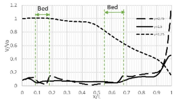
**Figure 11.** Graph of flow velocity distribution in a two-beds isolation room in the x-y plane ( $z=3$ )
