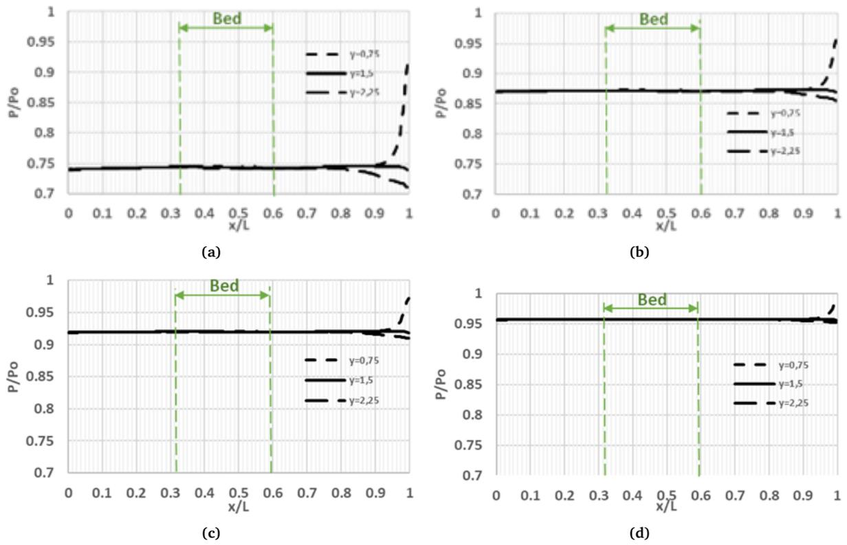
Figure 17. Graph of pressure distribution in a single-bed isolation room with variations of (a) -2.5 Pa, (b) -5 Pa, (c) -8 Pa, and (d) -15 Pa
