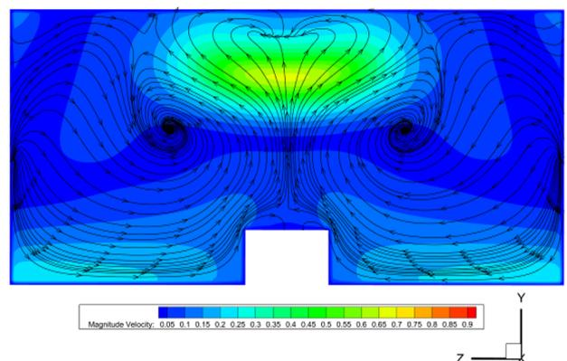
**Figure 6.** The contour of air velocity and streamline in a single bed isolation room in the z-y plane ( $x=4$ )
