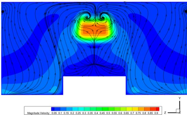
**Figure 8.** The contour of air velocity and streamline in a two-beds isolation room in the z-y plane ( $x=1.05$ )
