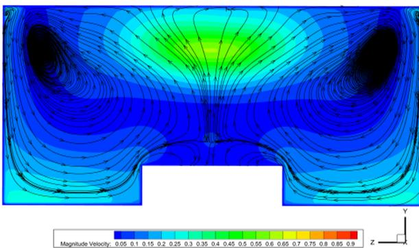
**Figure 9.** The contour of air velocity and streamline in a two-beds isolation room in the z-y plane ( $x=4.95$ )
