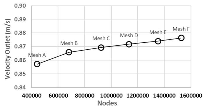
Figure 3. Grid independency test are related with velocity outlet
