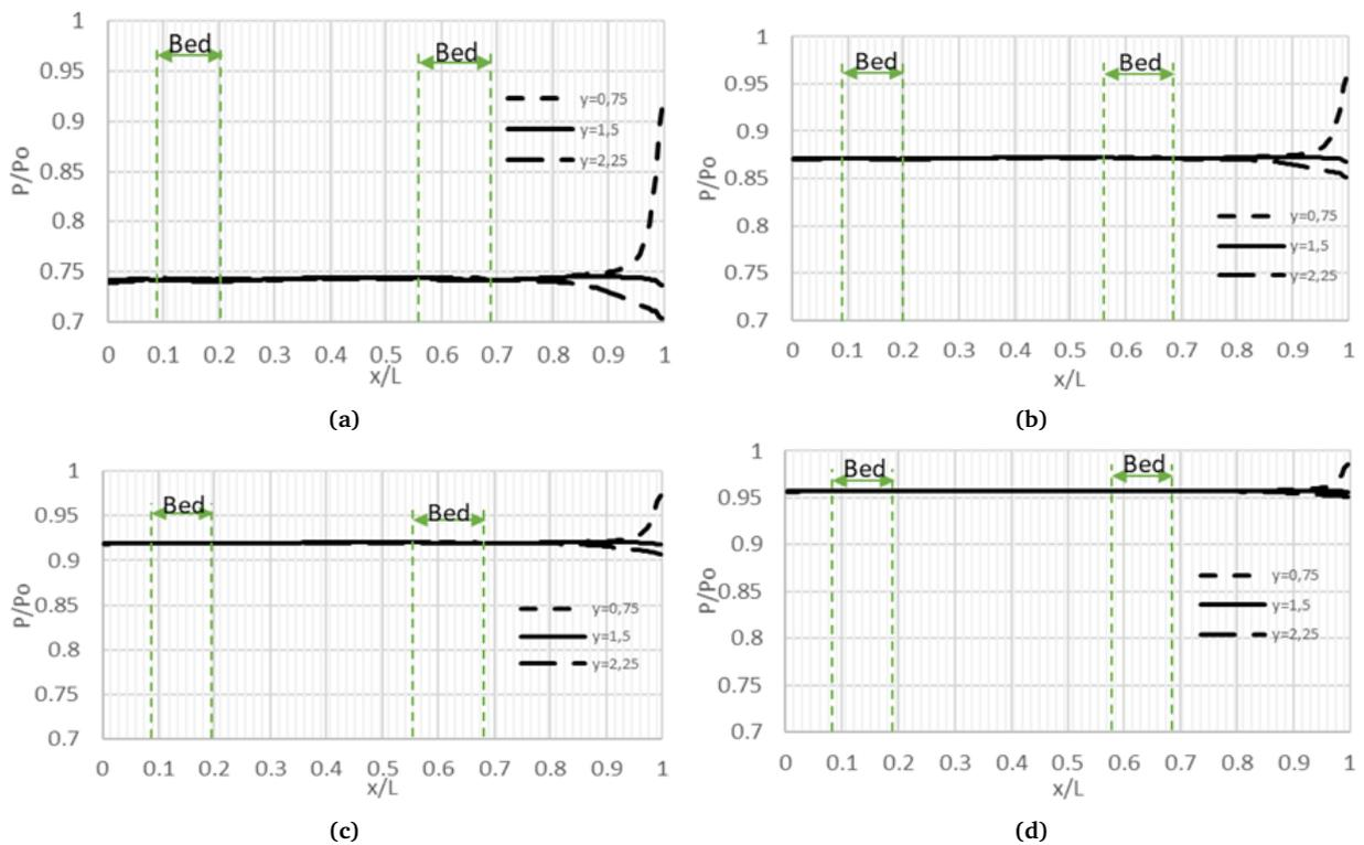
Figure 18. Graph of pressure distribution in a single-bed isolation room with variations of (a) -2.5 Pa, (b) -5 Pa, (c) -8 Pa, and (d) -15 Pa
