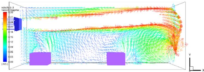
Figure 13. The flow vector in the two-beds isolation room in the x-y plane ( $z=3$ )
