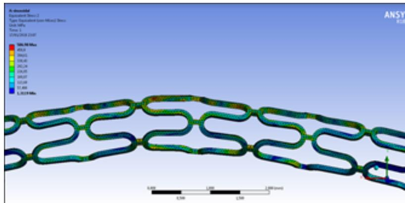
(a) Sinusoidal stent.
