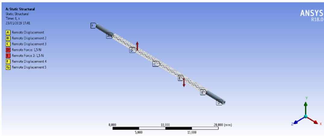
Figure 5. Load and boundary condition of stents and balloons.
