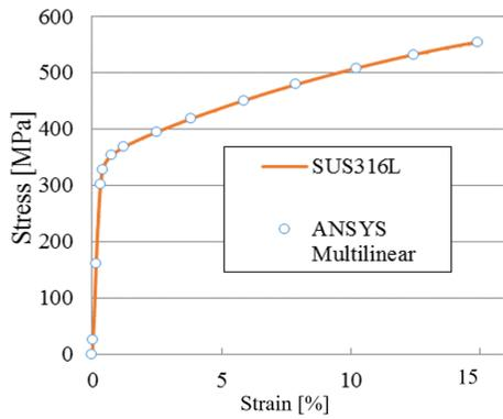
Figure 3. Fitting-test results of SS 316 L tensile test.
