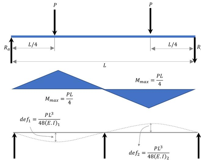
Figure 9. Load and deflection diagram.
