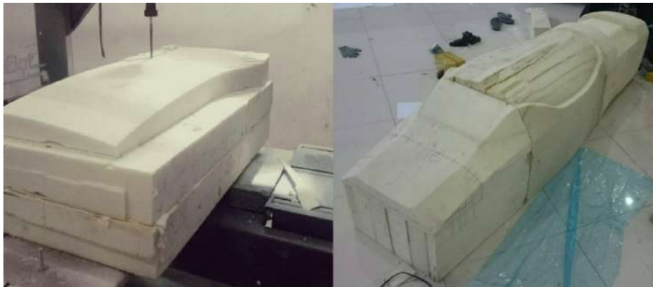
Figure 8. Master model making (a) machining, (b) positive model.
