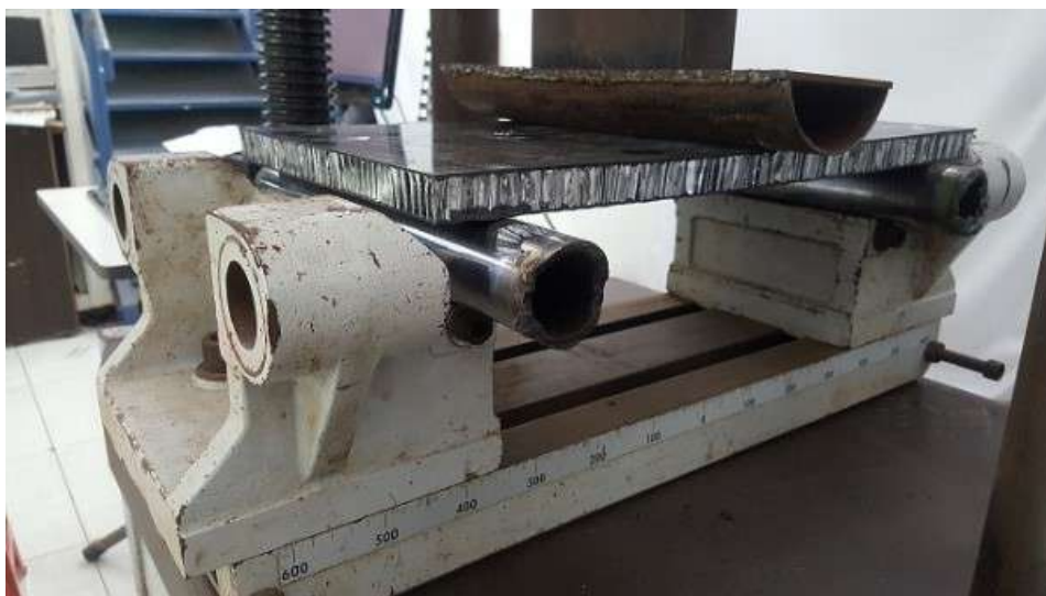
Figure 4. Specimen setup for 3-point bending experiment.
