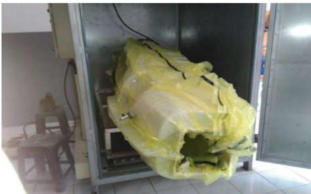
Figure 12. The curing process of the monocoque chassis.
