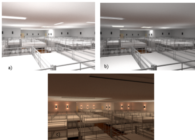
Figure 5. Passenger room lighting in conditions, a) in normal conditions, b) in emergency conditions, c) in sleeping conditions.
