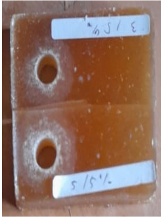
Figure 5. Casted polyester and rice husk composite specimens
