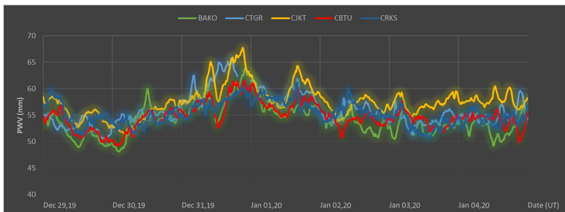
Figure 6.3. Time series of PWV values at 5 INACORS GNSS stations in the Jakarta flood area. The time spans from 29 December 2019 to 4 January 2020 (UT), and the highest PWV value occurred on December 31, 2019.
