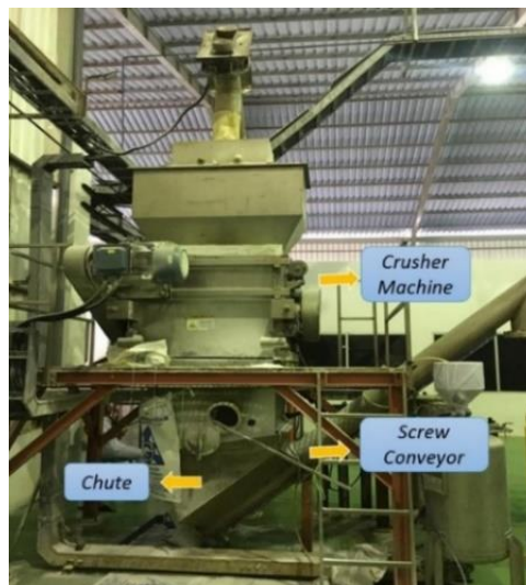
Figure 1. Crusher Machine II and Measurement of Wall Hopper
