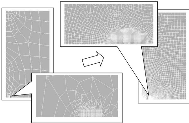
Figure 8. Composition of Elements Before and After Application of Element Size Control Modul
