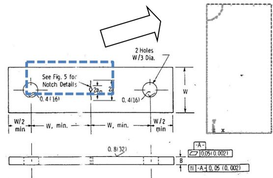
Figure 7. M(T) / CCT Standard Specimen (W < 75mm) (ASTM E647)
