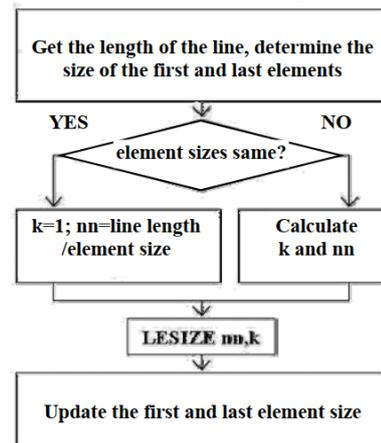
Figure 6. Flow of the Element Sizing Module
