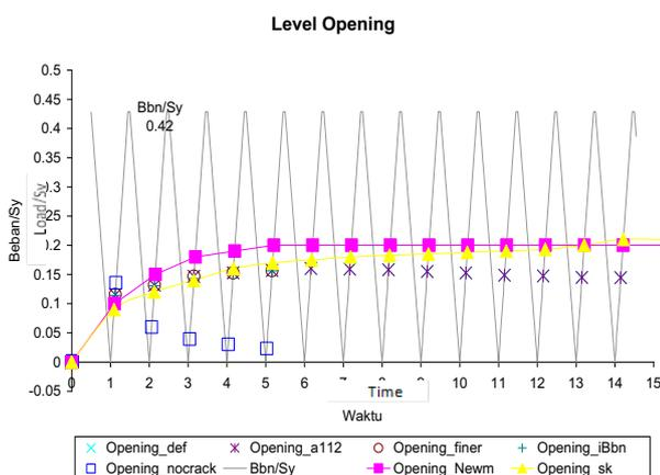
Figure 9. Comparison of Crack Opening Levels
