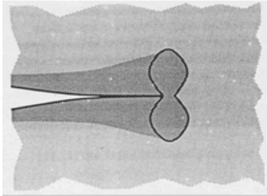
Figure 2. Early Crack Closure Due To Plasticity [10]
