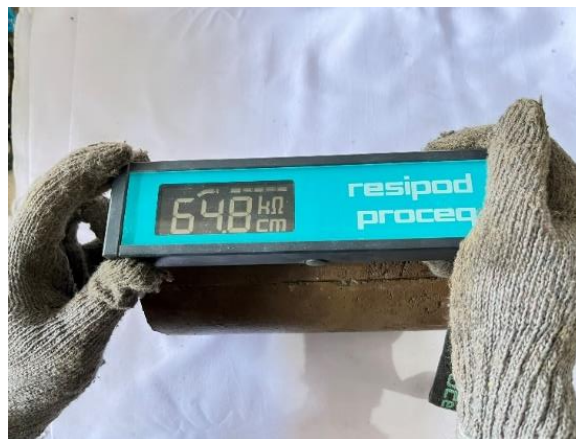
Figure 8. Resistivity Test Setup
