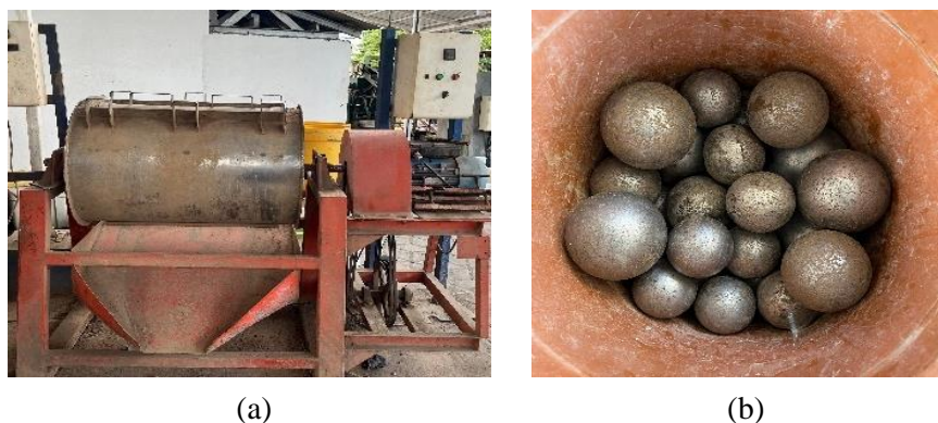
Figure 4. Dry Mixing Method Equipment, (a) Ball Mill Machine, (b) Iron Balls
