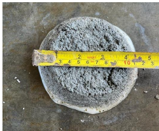
Figure 6. Flowability of Trial UHPC 0% Fly Ash 1% SP
