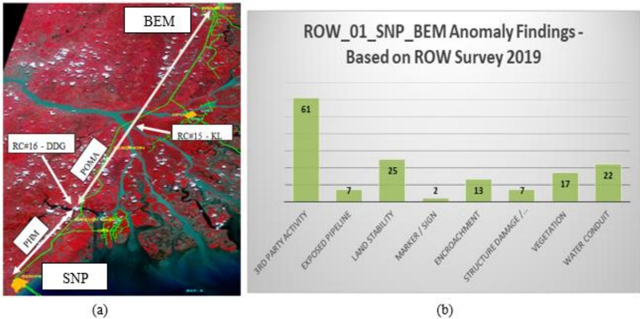
Figure 1. (a) Battery Limit of Pipeline Maintenance, (b) Anomaly Finding on ROW Survey 2019.
