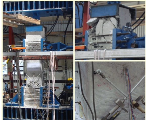
Figure 6. Failure of column specimen C-1RC
