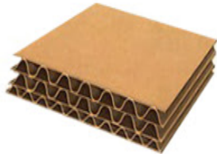
Figure 9. Corrugated Triple Wall
