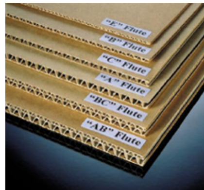
Figure 10. characteristics of each type of flute
