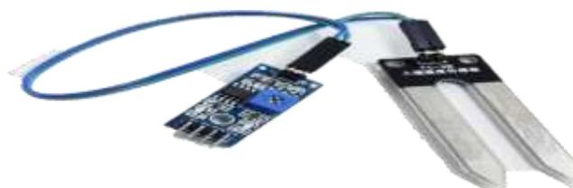
The YL-69 soil moisture sensor is an ideal sensor for monitoring city gardens or water levels in garden plants. This sensor consists of two probes for passing electric current in the soil as shown in
