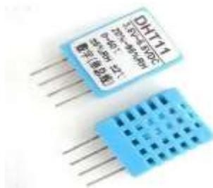
The DHT sensor in Figure 1 is a sensor that can measure air temperature and humidity. The working principle of DHT11 is like an NTC (Negative Temperature Coefficient) thermistor which utilizes changes in resistance when the temperature changes. The working principle of the DHT11 air humidity measurement is like the working principle of a capacitive sensor that utilizes changes in capacitance when there is a change in air humidity.
