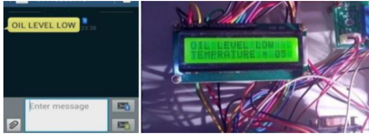
FIGURE 5 Oil Level Low Detection.
