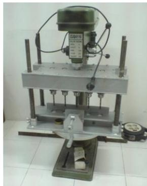
Figure 11. Gang Drilling Machine [9]
